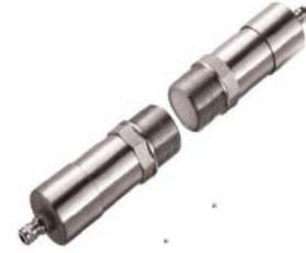
Microwave level detector provides a method of non-contact measurement, so it can be installed in silos, carrier pipes, rods or free fall extensions. According to different models, it can be applicable for a range of (0 ~ 8) m with customized wider range. For any vessel shell or carrier pipe of non-metallic materials, measurement can be directly conducted from the outside.
